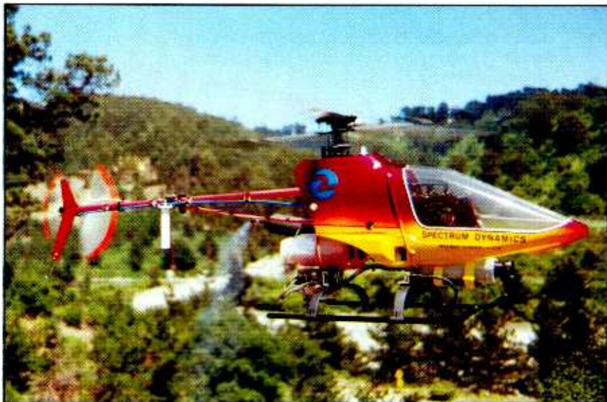
Side view of RPV ENG helicopter shows the camera beneath the cabin, the 2GHz transmitter located below the fuel tank and the omnidirectional ENG antenna on the boom near the tail rotor.
