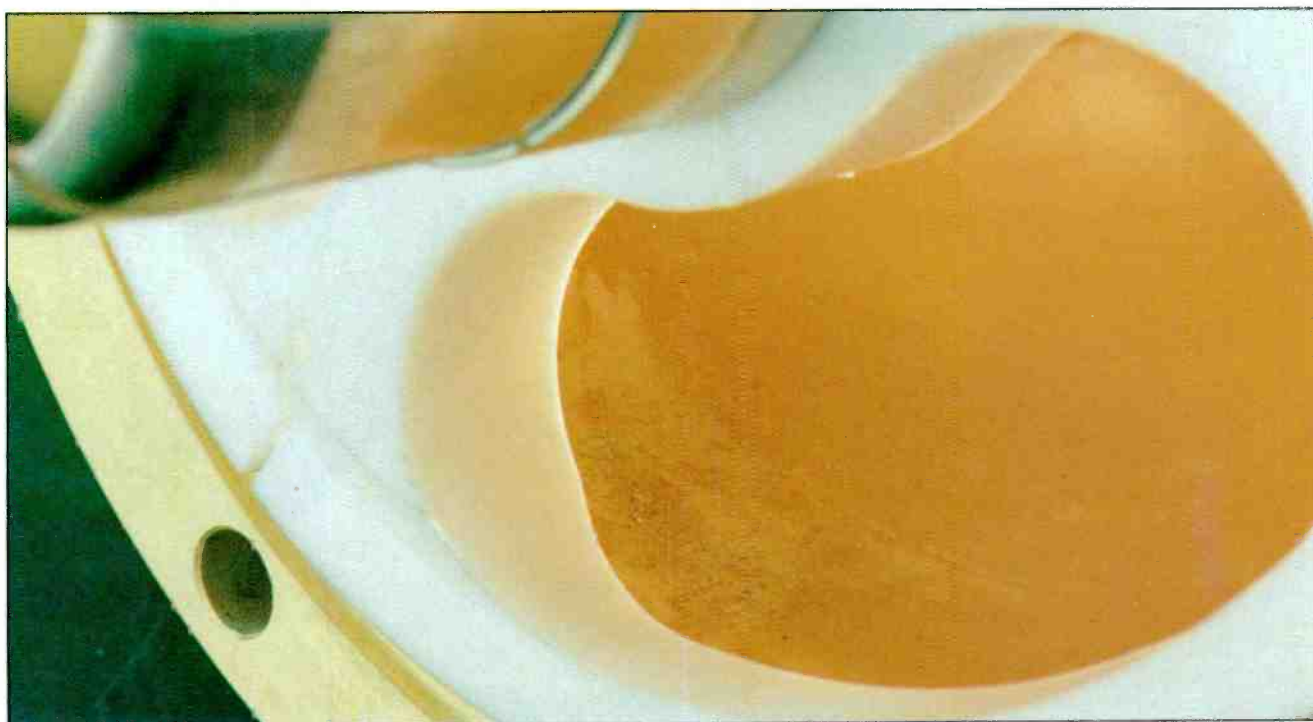
Figure 3. A look inside a horizontal outer conductor section, at metal shavings resulting from 10 years of simulated cyclic contraction/expansion (3,650 cycles) in a standard rigid transmission line.
