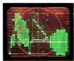
Triple Filter Parade— 1 H each of Flat, Low Pass and Chroma Filters
